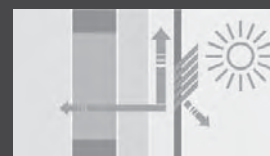
In summer, part of the heat is evacuated by circulating air
